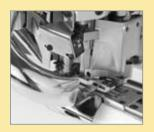
AK 气动切线装置+吸布屑组 pneumatic type chain cutter & waste suction set
